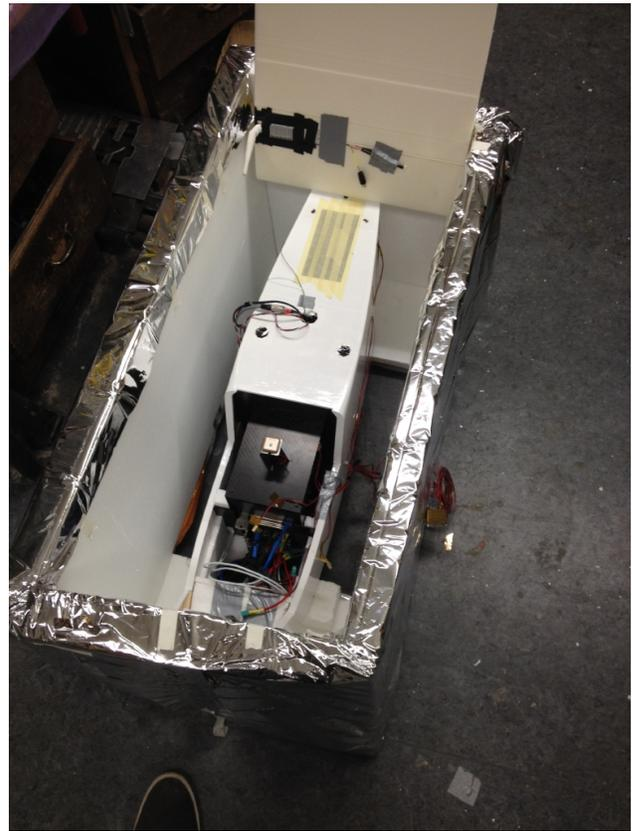
**Figure 11:** Fuselage with extra temperature sensors and video transmitter test setup
