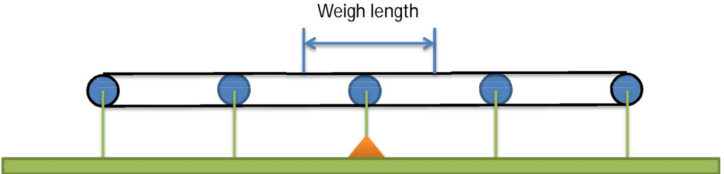
In case of two weigh bridges the weigh length is defined as follows:
