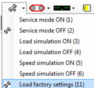
Concluding the factory defaults should be read in into SIWATOOL V7 via “Receive all data”:
