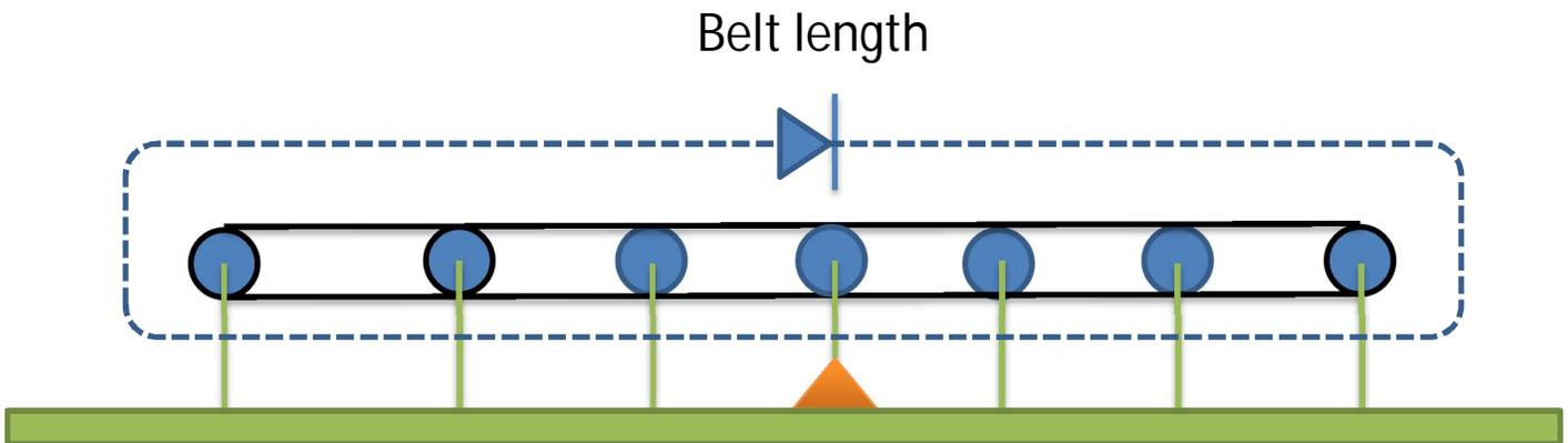
The unit for the belt length depends on the “Unit for belt load”. In case of “kg/m” it needs to be entered in meters, in case of “lbs/ft” it needs to be entered in feet.
