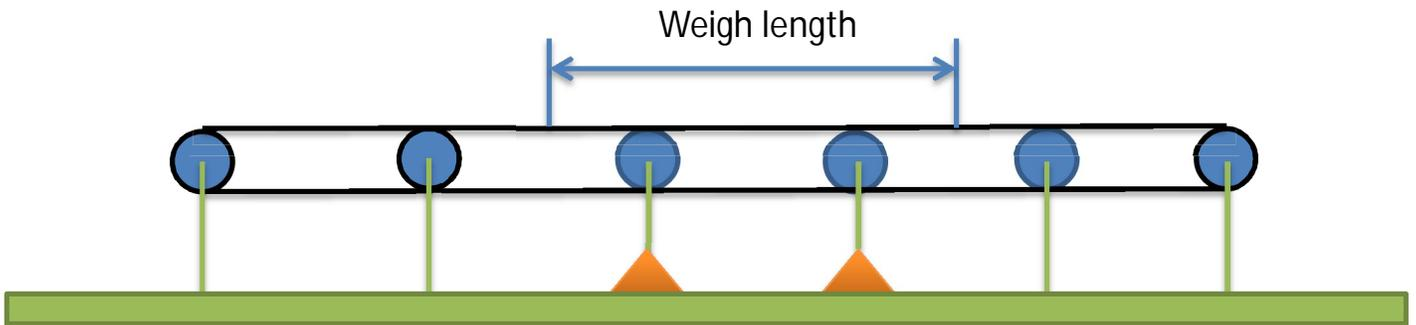
In case of three weigh bridges the weigh length is defined as follows:
