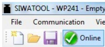
Once the connection was established, SIWATOOL V7 shows the connection status on the bottom on the right side (“Online” und a moving green bar):
