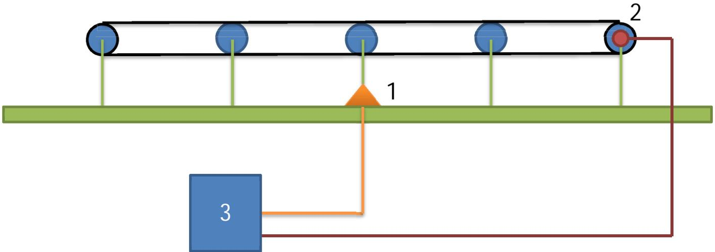
The integrator collects the load cells signal and the speed sensor pulses. With this information the actual belt load and belt speed can be calculated and multiplied with each other in order to get the current material flow rate on the belt. This flow rate is internally integrated in order to totalize the quantity of material conveyed over the belt.
