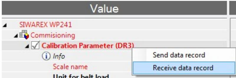
After that, all parameters of the corresponding data record are read into the "PC" column and therefore all parameters should be marked black afterwards, as there are no differences between online and offline data in the corresponding data record anymore.
