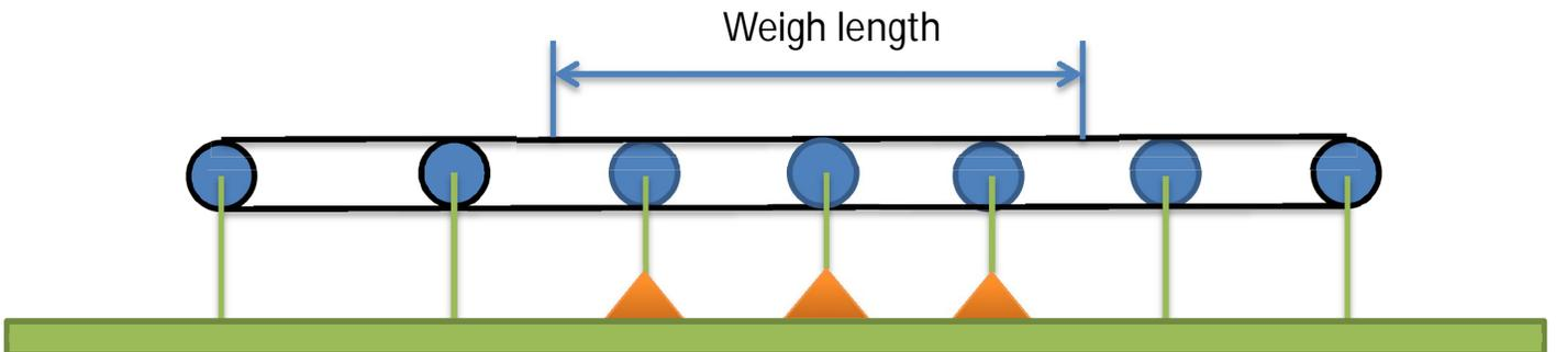
The unit for the weigh length depends on the "Unit for belt load". In case of "kg/m" it needs to be entered in meters, in case of "lbs/ft" it needs to be entered in feet.
