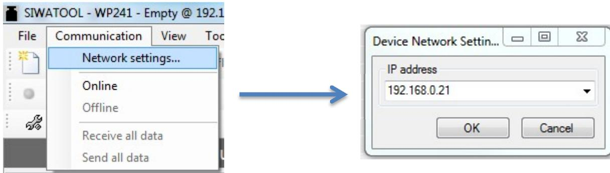
Factory default IP address of a SIWAREX WP241 is 192.168.0.21. The IP address of the PC Ethernet port needs to be in the same IP range like the WP241! As the WP module supports auto negotiation, a basic Ethernet patch cable can be used for a direct connect from PC to the WP module.
