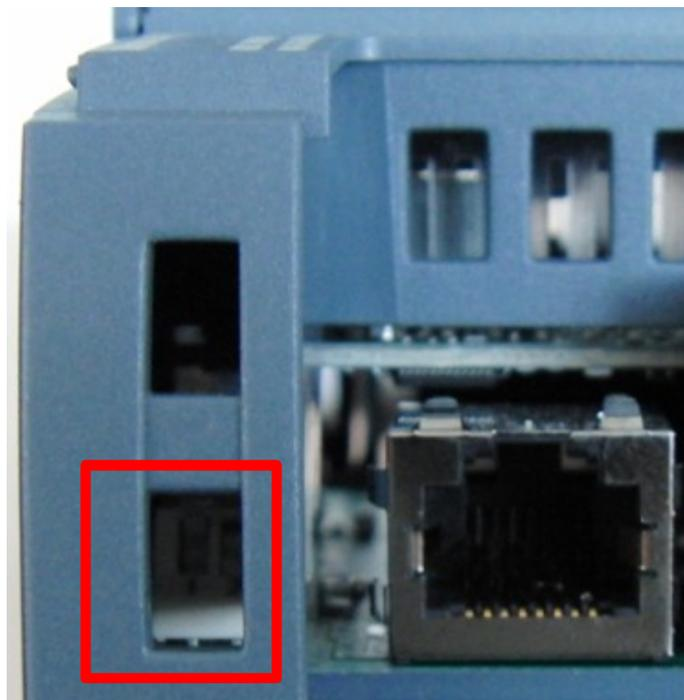
The DIP switches are located left beside the Ethernet port of the WP241. By using a small screw driver, the device can be set to stand-alone operation. As factory default the right DIP switch (DIP no. 2) is in upper position (= integrated S7-1200 mode). Set this switch to the lower position for stand-alone operation. After that the 24V can be connected to start up the WP241.
