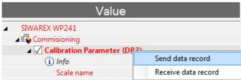
After that, all parameters of the corresponding data record are written from the "PC" column into the WP241 (= into the "SIWAREX" column) and therefore all parameters should be marked black afterwards, as there are no differences between online and offline data in the corresponding data record anymore.
